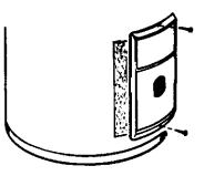
3. Open the flap of insulation to expose the opening.
